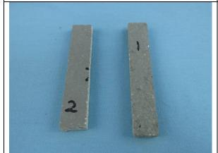
Reference sample Tested sample 10%(m/m) AC-3 CIP Acid Cleaner
