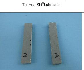
Reference sample Tested sample 10%(m/m) Tai Hua Shi <sup>®</sup>SPARTEC Quaternary Ammonium Salt Disinfectant
