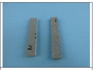
Reference sample Tested sample 10%(m/m) TOPAX 19 Alkaline Foam Cleaner
