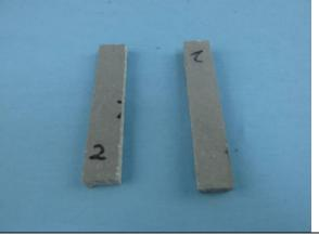
Reference sample Tested sample 10%(m/m) SU 626 Heavy Duty Foam Gel Cleaner
