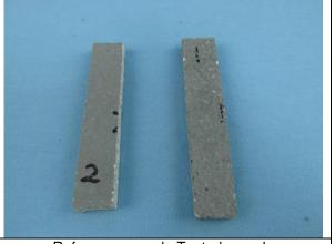
Reference sample Tested sample 10%(m/m) Bottle Additives YI XI YANG A
