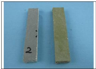
Reference sample Tested sample 12% (m/m) Sodium Hypochlorite
